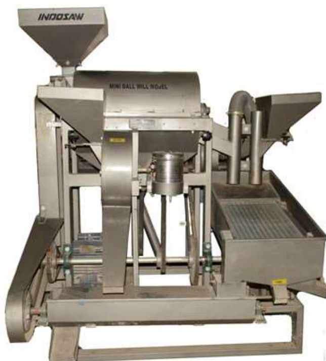
Fig. 1: PDKV Dal mill used in the study for milling of selected pulses
