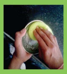
Caption: The bars are made to undergo tests to check their capacity to clean tough soil as also for any scratch that may be left on the dish
