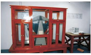
Reference Standard equi-arm double pan balance in reference Standard Laboratory
