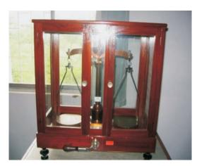
Working Standard equi-arm double pan balance in Working Standard Laboratory
